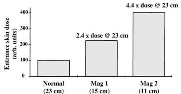
**Figure 5.** Effect of electronic magnification on entrance skin dose. The radiation dose increases by the square of the ratio of the image intensifier diameters. *arb* = arbitrary, *Mag* = magnification.
